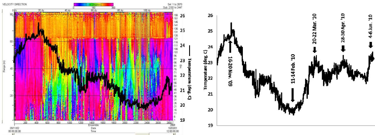
Figure 4: (left) Unprocessed current direction in degrees relative to North measured with the bottom mounted ADCP deployed in the Tortuga navigation channel; water temperature measured at the bottom mount location is overlaid in black in degrees Centigrade. (right) Water temperature at ~68 m depth measured with a SBE 39 deployed with the bottom mount.
